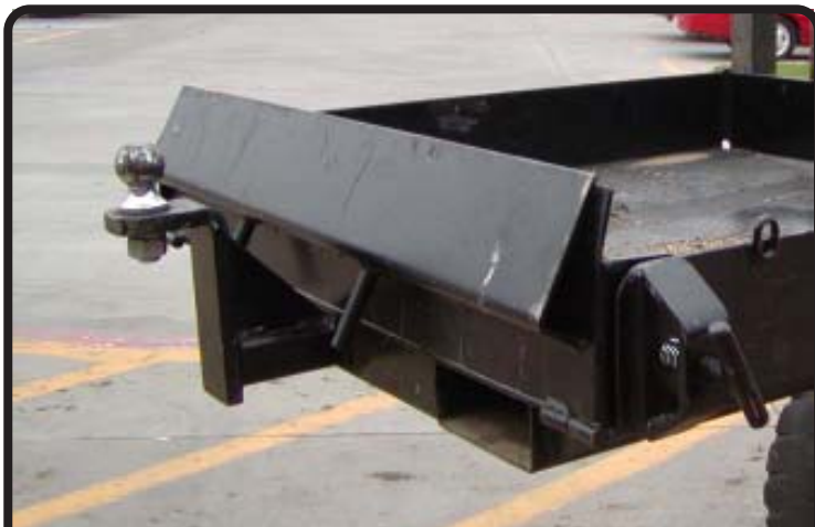
Built-in receiver for moving trailer mounted equipment. Accepts standard 2" sq. trailer adapter. (Shown with optional adapter and ball.)
